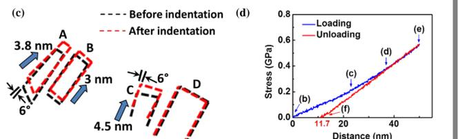
In situ nanoindentations on TiN thin film with 20 nm grain size show a lot of grain activities, including grain rotation and boundary sliding, some of which are irreversible. Stress-displacement plot shows significant inelastic deformation behavior.
