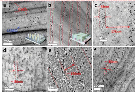
Rectangular  $\text{CeO}_2$  pillars are strongly confined and aligned in one-direction and formed ordered  $\text{CeO}_2$  rows in LSMO matrix, random while distribution of the circular  $\text{CeO}_2$  pillars/domains without any obvious long-range order has been observed on untreated STO.
