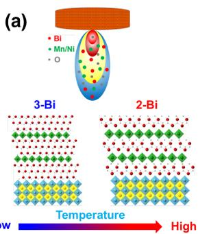
Tunable layered structures have been achieved by precisely controlling the growth conditions.
