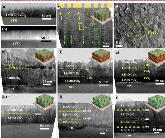
Microstructure of the designed 3-D VAN structures
