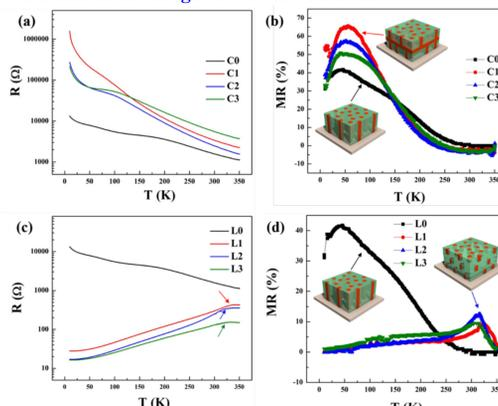
Samples with  $\text{CeO}_2$  interlayer show typical semiconductor behavior, while samples with LSMO interlayer show metallic behavior, from the RT results; MR% of film C0-C3 increase firstly and then reduce as the temperature rises from low temperature to room temperature; L1-L3 structures enables higher MR values at higher temperature, e.g., 13% at 316 K in sample L2.
