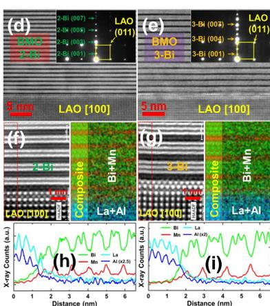
The structure of Bi-Mn-O based layered supercell can be controlled by the growth conditions.
