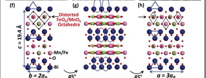
BFMO film on the pseudo-perovskite  $\text{LaAlO}_3$  (001) substrate shows a supercell (SC) structure along the  $c$ -axis. Graphic phase analysis shows a highly strained transition layers between substrate and SC. An atomic model of the novel BFMO phase with  $a = 2a_p$  ( $a_p \sim 3.99 \text{ \AA}$  stands for the lattice parameter of the pseudo-perovskite BFMO),  $b = 3a_p$  and  $c \sim 19.40 \text{ \AA}$  is proposed based on the STEM images.
