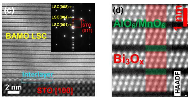
The Bi-Al-Mn-O layered supercell is composed of alternative layered stacking of  $\text{Bi}_3\text{O}_x$  and Al/Mn-O octahedral slabs along the film growth direction.
